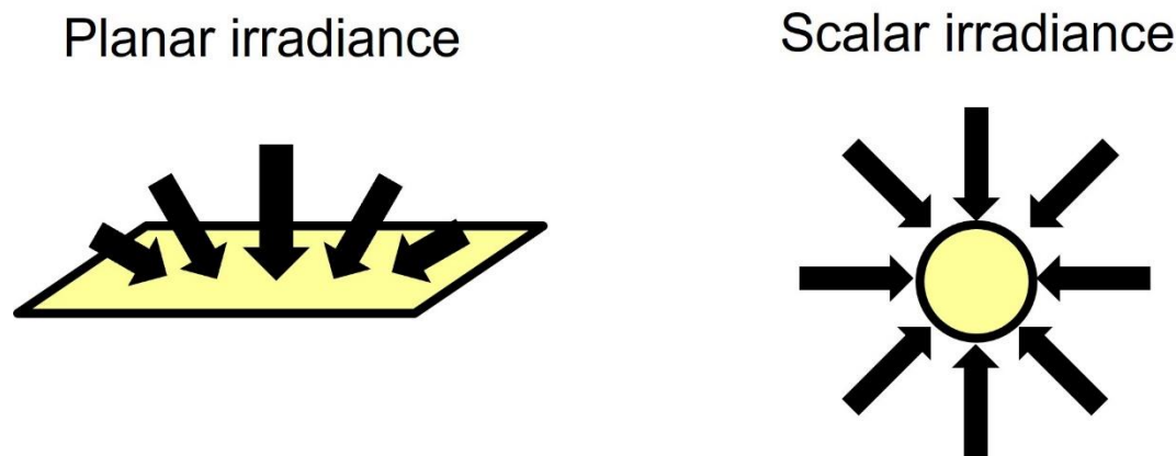
Figure S1: Planar irradiance (light incident on a flat surface with cosine weighting) and scalar irradiance (light incident on a sphere or point in space with no angular weighting). Sketch A. Jechow
